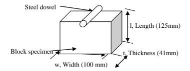
Figure 3: Shows the specimens configuration. These methods were applied to determine the WBCSD as shown in Figure 4.
