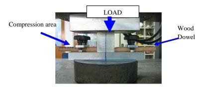
Figure 6: Test Set-up of WDCSB
