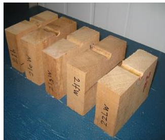
Figure 2: Bearing strength specimens ready for test
