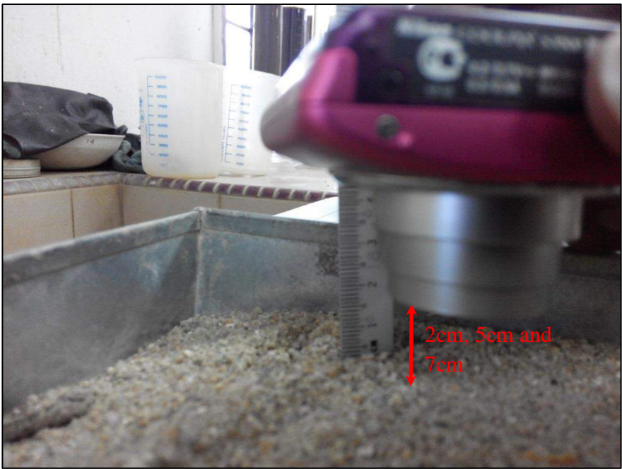
Figure 4: Distance between camera lens and sample
