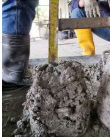
Figure 6: Slump test results
