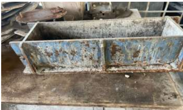
Figure 3: Beam mould 150 x 150 x 500m
