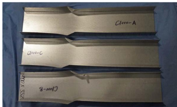
Figure 2: The Failed Specimens with 1 Meter Long
