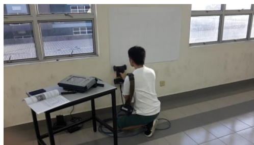
Figure 3: GPR Scanning On Area 1 (Wall)
