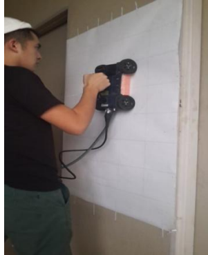
Figure 8: GPR Scanning On Area 6 (Column)
