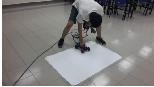
Figure 4: GPR Scanning On Area 2 (Floor)
