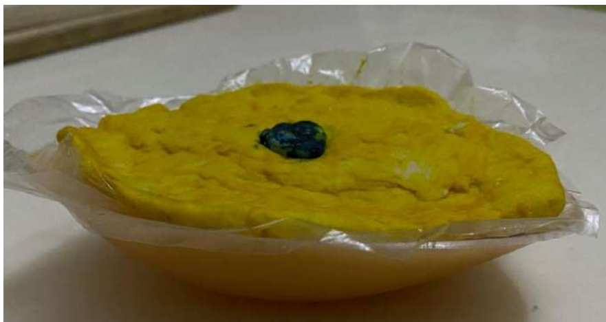
Figure 7: Developed homogenous breast phantom with tumour
