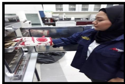
Figure 2: Placing the Mangifera Indica Seed to the oven for 24 hours
