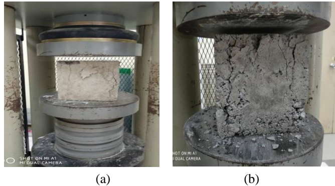
Figure 3: Compressive Strength Test (a) Before Compress, (b) After Compress
