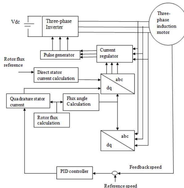
Figure 1: Overall Block Diagram of the Proposed Design
