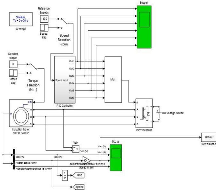
Figure 3: Developed SIMULINK model for the proposed PID controller of Three-Phase Induction Motor
