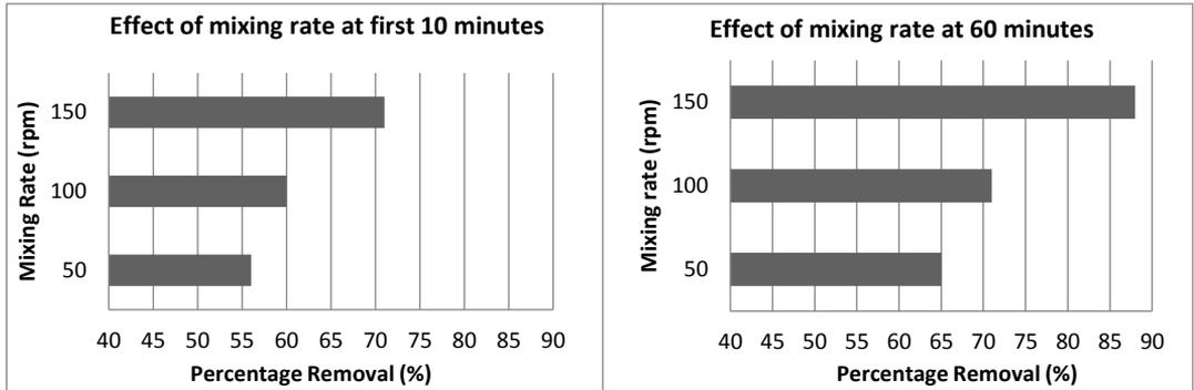
Figure 5: Effect of mixing time on the uptake of Fe (II) ions by durian leaves at the first 10<sup>th</sup> minute and 60<sup>th</sup> minute
