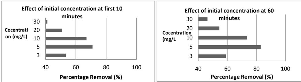
Figure 3: Effect of initial Fe(II) ion concentration and contact time on the uptake of Fe(II) ions by durian leaves in the first 10 minutes and 60<sup>th</sup> minutes
