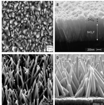
**Figure 1: SEM figures: (a) the SnO<sub>2</sub>:F surface of the conducting glass substrate, (b) ZnO layer deposited by spray pyrolysis on conducting glass, (c) planar view (45° tilted) and (d) cross section of electrodeposited ZnO(20 c cm<sup>-2</sup>) on a glass /SnO<sub>2</sub>:f / ZnOSP sample [30]**
