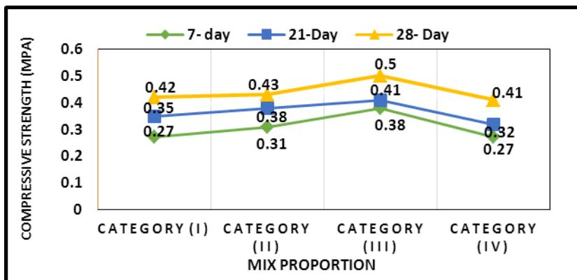
Figure 5: Compressive Strength Test of Control Sample
