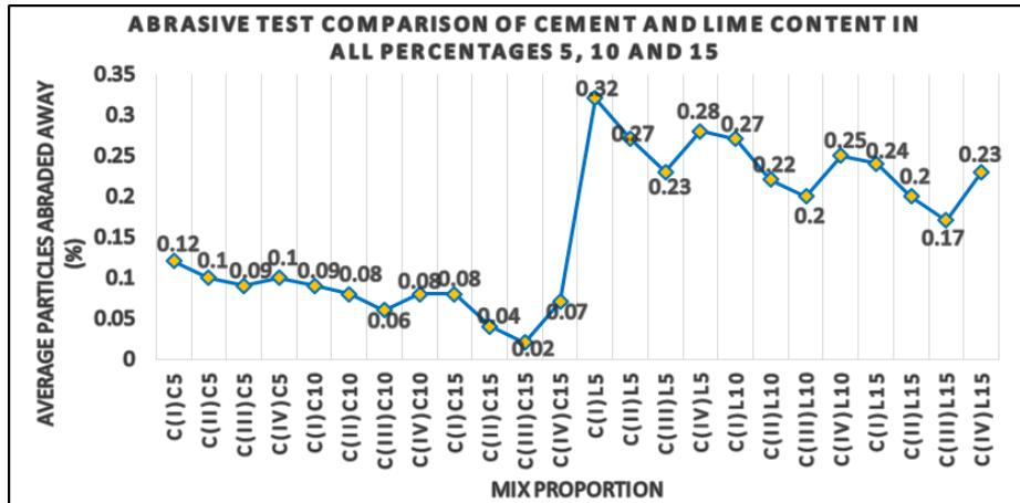
Figure 9: Abrasive Test of Specimen without Stabiliser
