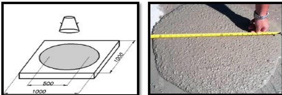
Figure 7: Slump Flow Test (BS EN 12350-8:2010)
