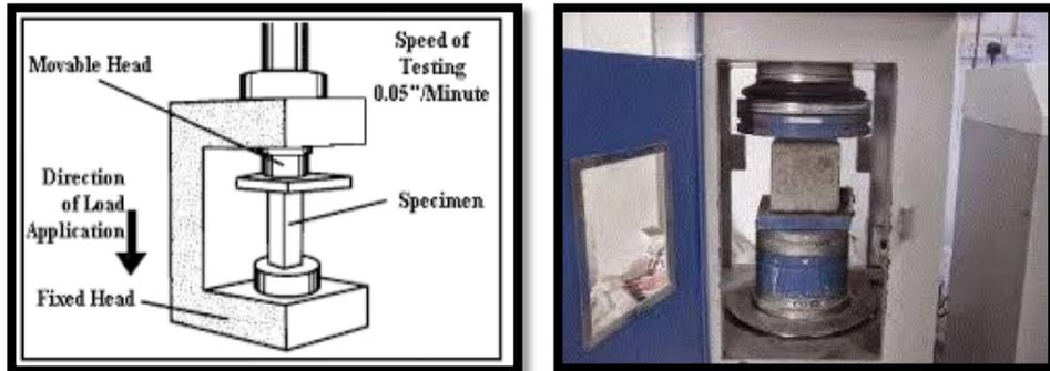
Figure 8: Compressive Strength (BS EN 12390 – 3: 2009)
