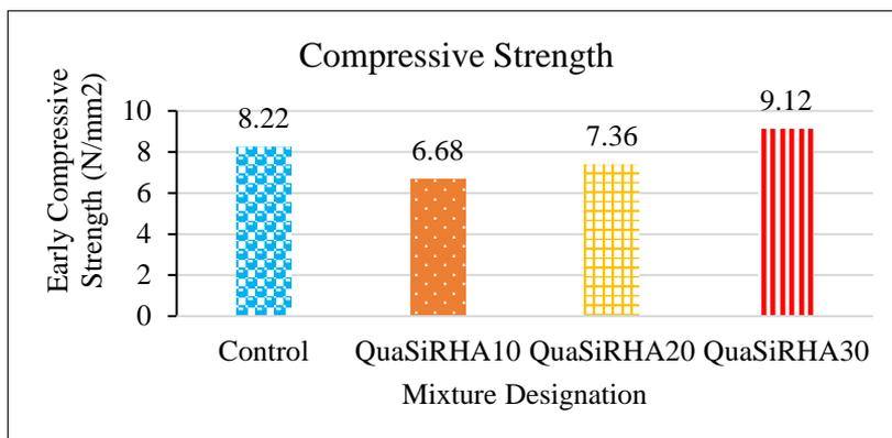
Figure 10: Compressive Strength of Concrete Mixture Design
