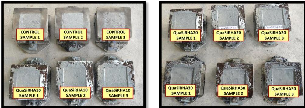
Figure 6: Concrete specimens for control, QuaSiRHA10, QuaSiRHA20, QuaSiRHA30
