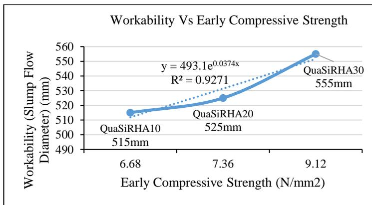
Figure 11: Workability vs Strength of Concrete Mixture Design
