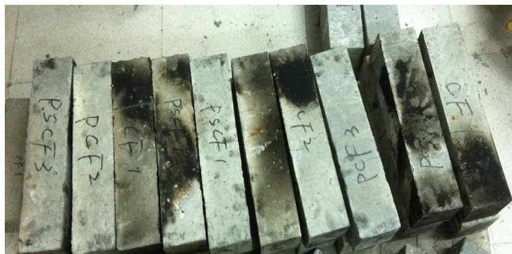
Figure 4: Appearance of the concrete test block after being exposed to fire
