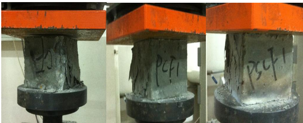
Figure 5 Destruction patterns of benchmark concrete, single-polypropylene fiber concrete and hybrid fiber concrete after compression
