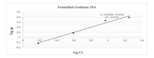
Figure 9: Freundlich Isotherm Plot for the Adsorption of Zinc Ions onto Papaya Seed
