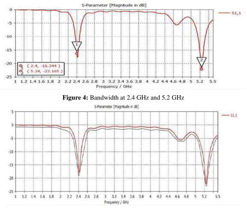
Figure 5: Difference between simulated and measured Return loss
