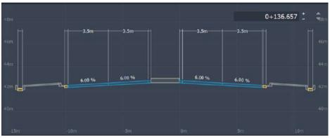
Figure 8: Cross Section of Road on Bridge
