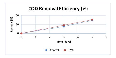
Figure 2: COD Removal Rate of Conventional and Modified CSTR.
