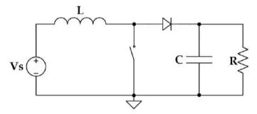
Figure 3: Schematic diagram for boost converter.
