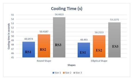
Figure 11: Cooling time (s) in comparison with runner in round shape and elliptical shape
