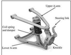
Figure 3. The double-wishbone suspension system (Arikere, A., Saravana Kumar, G., & Bandyopadhyay, S. (2010)).
