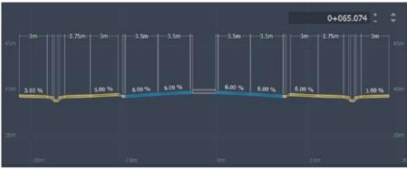
Figure 6: Cross Section of Road Design on Ground
