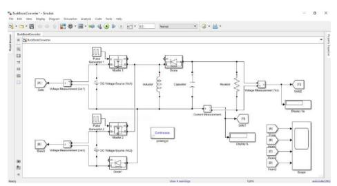
Figure 11: Multiple input buck-boost converter circuit using MATLAB
