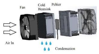
Figure 2: Working principles of Peltier Dehumidifier
