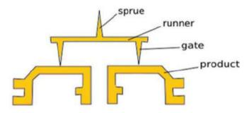
Figure 3: Sprue, runner and gate diagram. (Mehdi, 2019)
