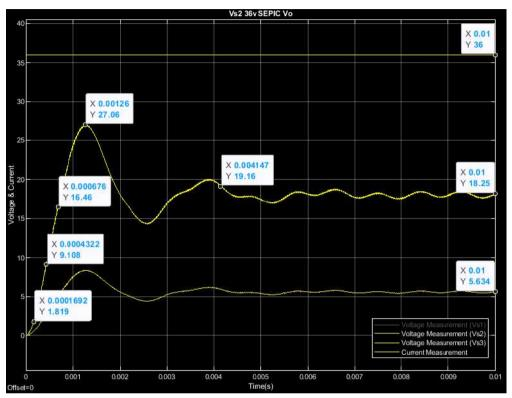
Figure 15: SEPIC output voltage when voltage source 2 active only.
