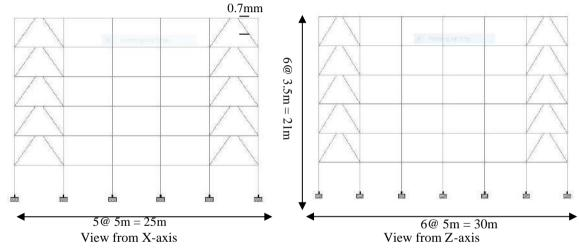
Figure 4: Elevation view of the Frame B (EBF)
