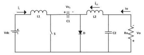
Figure 8: Schematic diagram for Cuk converter.
