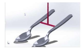
Figure 7: Two cavities of disposable spoon in the mould design
