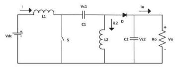
Figure 9: Schematic diagram for SEPIC converter.
