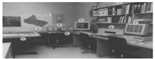
Figure 2 : Typical GIS Laboratory with Components: (1)Scanner; (2)Digitizing Table;
