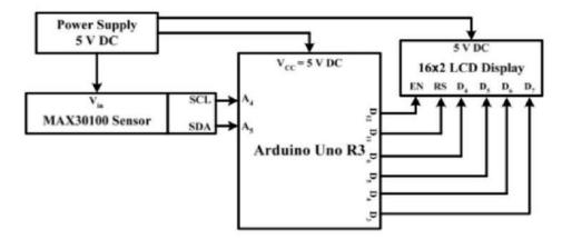
Figure 2.5: Block Diagram of Oxygen Saturation Measurement System [5]
