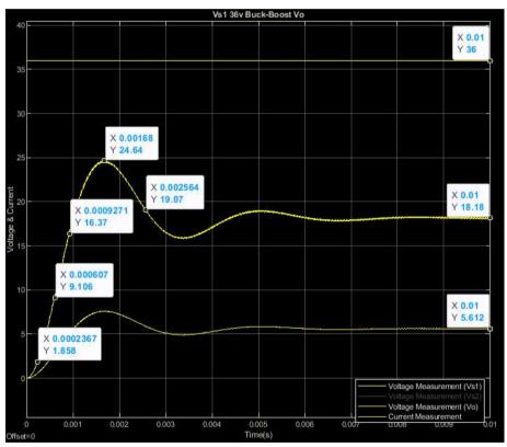
Figure 13: Buck-boost output voltage when voltage source 1 active only.
