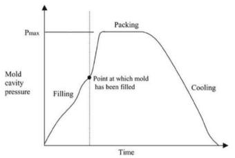
Figure 2: Pressure along the processes (Zhou, 2013)
