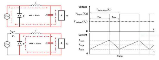
Figure 2: Buck converter circuit and characteristic.
