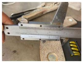
Figure 5: Clutch Plate Inner Diameter (Aftermarket)
