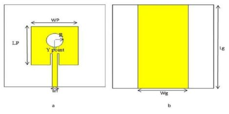
Figure 1: Geometric design of the proposed antenna
