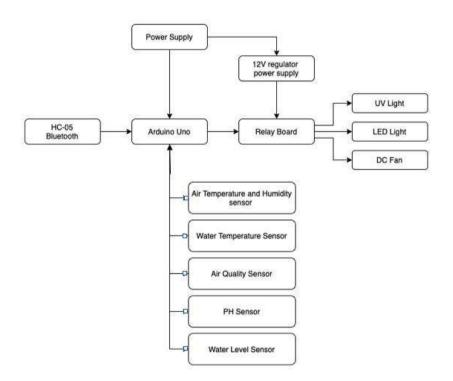
Figure 2: Overall Block Diagram of the Proposed Design
