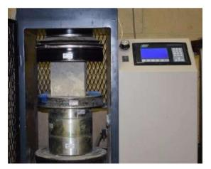
Figure 4: Compression test setup and the instrumentation.
