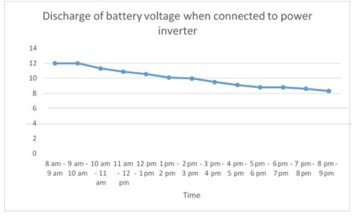
Figure 8: Discharge of battery voltage
