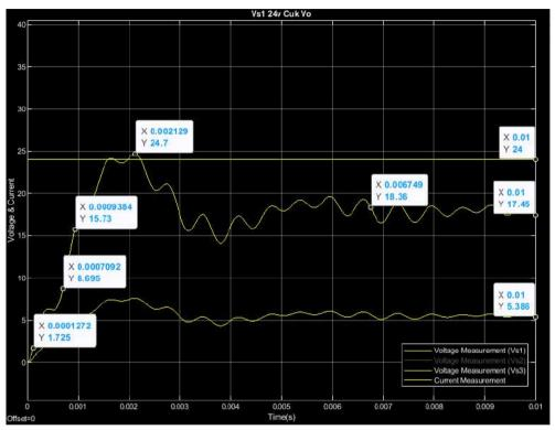
Figure 18: Cuk output voltage when voltage source 1 active only.
