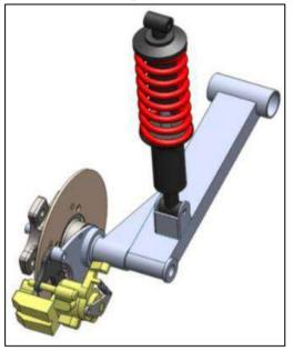
Figure 4: The trailing arm suspension system. (Huang, H. H., & Chen, S. L. 2019).
