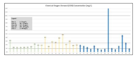
Figure 4-4: COD Concentrations of all water samples extracted
