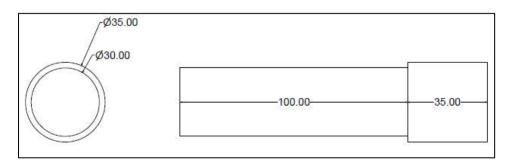
Figure 3: Workpiece sample dimension
