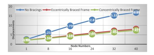
Figure 6 is a graphical representation of the nodal displacements due to the seismic load acting along the x-axis of the three frames for six nodes which I selected to make the
