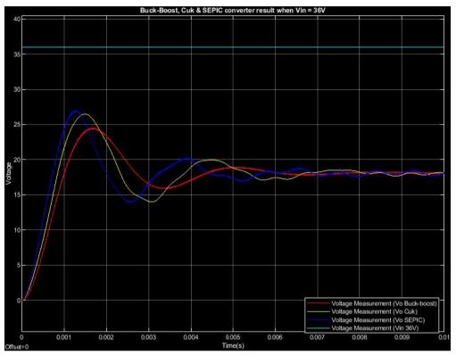
Figure 16: Different types of converter result when input is 36 V.
