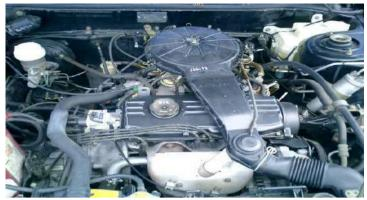
Figure 1: Proton Iswara 4G13 Engine System
