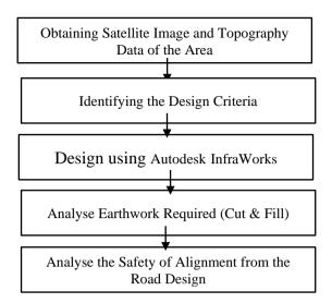
Figure 2: Flow Chart of Route Design using Autodesk InfraWorks
