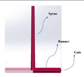
Figure 6: Feed system designed in CAD
