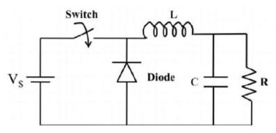
Figure 1: Schematic diagram for buck converter.
