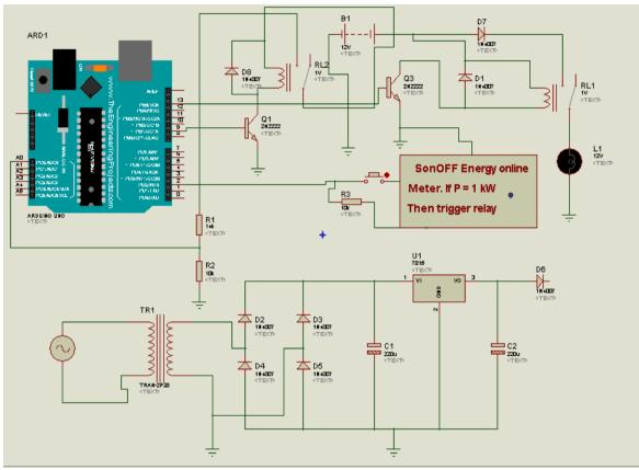
Figure 1: Peak shaving schematic diagram
