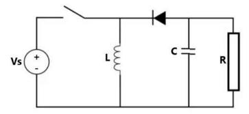
Figure 5: Schematic diagram for buck-boost converter.
