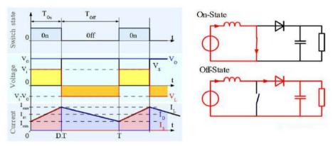
Figure 4: Boost converter characteristic and state of circuit.
