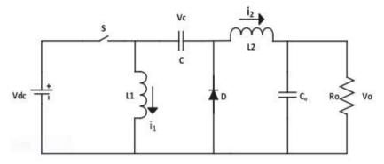
Figure 7: Schematic diagram for zeta converter.
