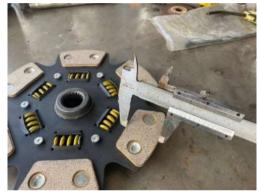
Figure 6: Clutch Plate Contact Surface Area (Aftermarket) Table 3: Properties of Different Materials
