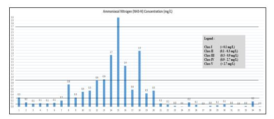
Figure 4-5: NH3-N Concentrations of all water samples extracted
