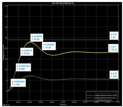
Figure 17: Buck-boost output voltage when voltage source 2 active only.
