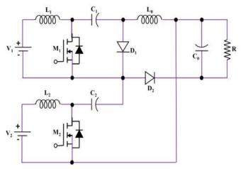
Figure 10: Fused Cuk-SEPIC converter equivalent circuit.
