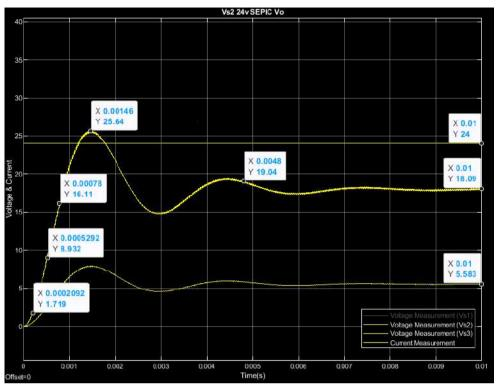
Figure 19: SEPIC output voltage when voltage source 2 active only.
