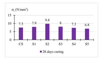
Figure 11: Average tensile strength on day 28
