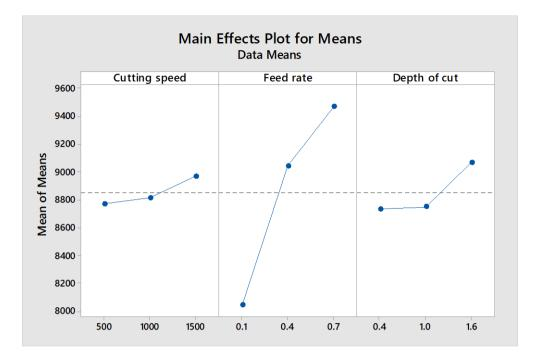
Figure 9: Main Effects Plot for Means for MRR
