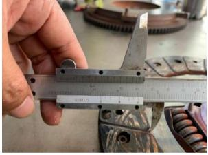
Figure 3: Clutch Plate Inner Diameter (Conventional)
