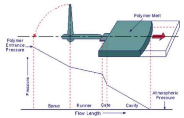
Figure 1: Pressure decrease along the feed system, (Zhou, 2013)
