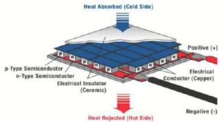
Figure 1: A Cutaway of Thermoelectric Module [3]
