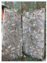
Figure 9: The damaged concrete cylinder after the split tensile test.
