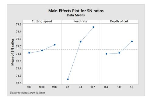
Figure 8: Main Effects Plot for S/N Ratios on MRR
