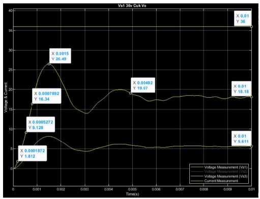
Figure 14: Cuk output voltage when voltage source 1 active only.
