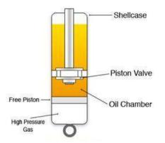
Figure 2: Monotube Shock Absorber (Johnny, 2016)
