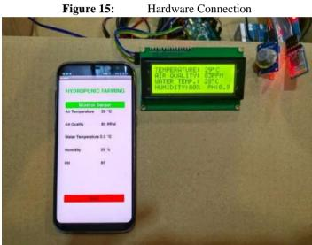
Figure 16: Monitoring of temperature, air quality, water temperature, humidity and pH value.
