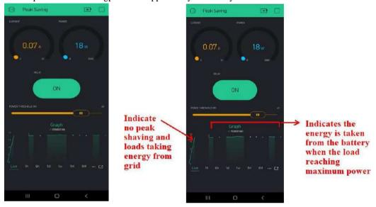
(a) Peak shaving captured during the operating of automatic switching (b) Explanation on peak shaving system
