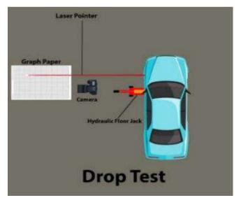
Figure 9: Set-up planning at experimental site with measuring tool
