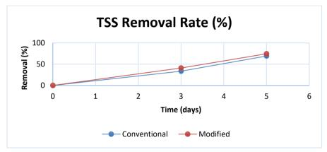
Figure 3: TSS Removal Rate of Conventional and Modified CSTR.
