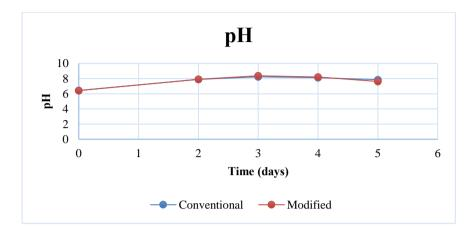
Figure 1: pH of Modified CSTR and Conventional CSTR.
