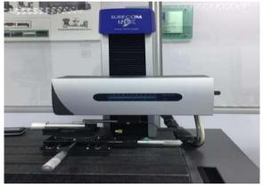
Figure 4: Surfcom Nex for Ra Measurement
