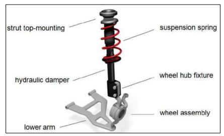
Figure 5: Schematic view of a McPherson front strut suspension system Czop, P. (2011)
