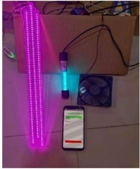
Figure 17: LED Light, UV Light and DC Fan
