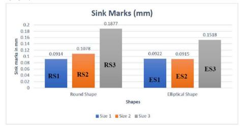
Figure 12: Sink marks (mm) in comparison with runner in round shape and elliptical shape
