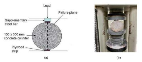
Figure 8: Test setup for split tensile test and instrumentation (a) schematic (b) experimental.
