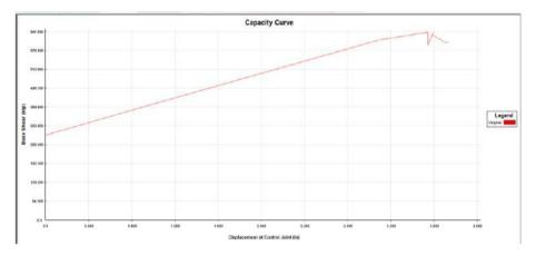
Figure 10: Capacity Curve for Concentrically Braced Frame
