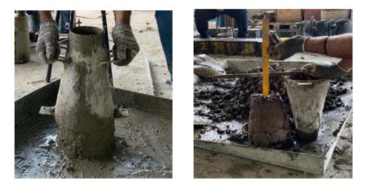
Figure 3: Slump test setup and procedure.
