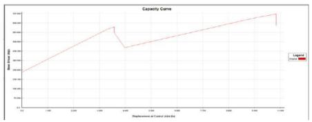
Figure 8: Capacity curve for Steel Frame without Bracings
