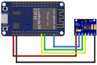
Figure 2.6: Interfacing MAX30100 with ESP32 [6]
