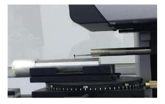
Figure 5: Setup of Surfcom Nex for Measurement of Ra
