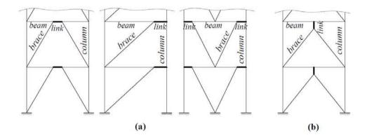
Figure 1: (a) Horizontal links: K frame; D frame; V frame; (b) Vertical links (Y frame)
