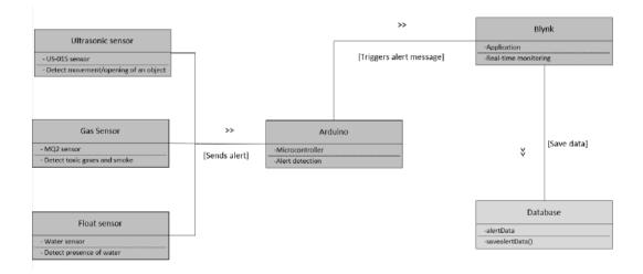
Figure 1.12: Conceptual Class Diagram
