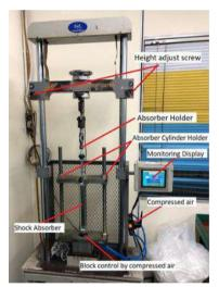
Figure 7: Shock absorber tester MST-10kN
