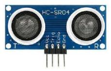
Figure 1.3: Ultrasonic sensor
