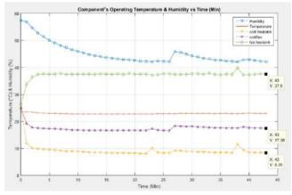
Figure 10: Component's temperature and humidity value after the experiment at indoor condition with relay and without heater.
