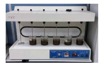
Figure 4: Mixing using jar test
