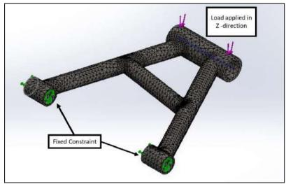
Figure 6: Boundary condition for numerical study.
