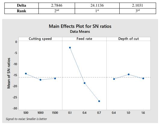
Figure 6: Major Effect graph for Signal to Noise Ratios for Ra (Smaller-the-Better)
