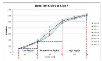
Figure 15: Regions of Damping Coefficient of the Shock Absorber Click 0 to Click 7
