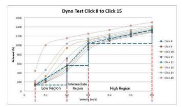
Figure 16: Regions of Damping Coefficient of the Shock Absorber Click 8 to Click 11
