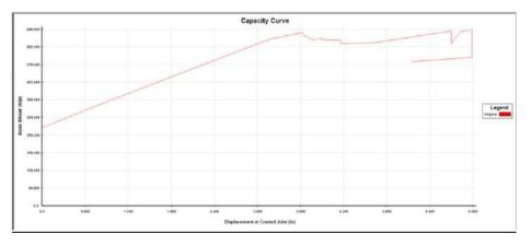
Figure 9: Capacity curve for Eccentrically Braced Frame
