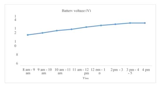
Figure 4: The plot of 12 V battery charging voltage
