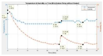
Figure 9: Temperature and humidity value after the experiment at indoor condition with relay and without heater.
