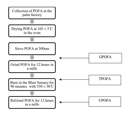
The next step was burning the POFA at  $550 + 50^{\circ}$ C in a gas furnace. The result as in the figure 3.3. This is to remove excess unburnt carbon. Lastly the POFA was again grind in a ball mill for 12 hours to obtain the ultrafine POFA and also to ensure the uniformity and consistency of the ultrafine POFA
