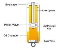
Figure 1: Twin Tube Shock Absorber (Johnny, 2016)
