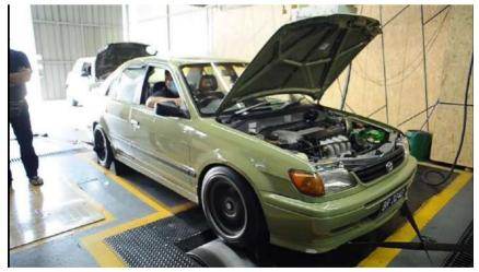
Figure 2: Vehicle Strapped on Chassis Dynamometer
