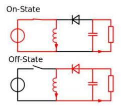
Figure 6: Buck-boost converter state of circuit.
