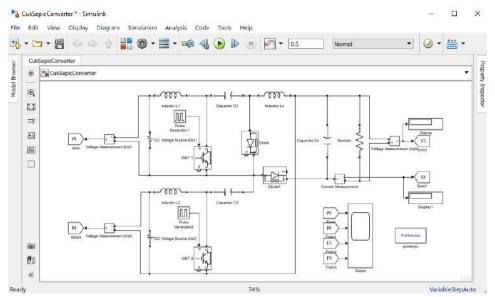
Figure 12: Multiple input Cuk-SEPIC converter circuit using MATLAB
