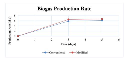
Figure 5: Biogas Production Rate of Conventional and Modified CSTR.
