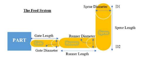
Figure 5: Schematic diagram of feed system
