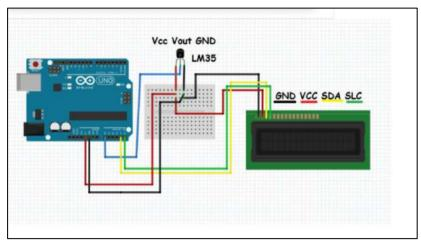
Figure 2: Temperature measuring system schematics
