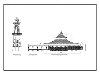
**Figure 2**: The roof of Masjid Jamek Seremban is unique as it concurs with the style of Malaccan Architecture. The most striking feature of the roof is its style, a multi-tiered pyramidal roof. Each tier of the roof has an opening made of stained glass. The stained glass offers a unique opportunity for ventilation while simultaneously providing natural sunlight.
