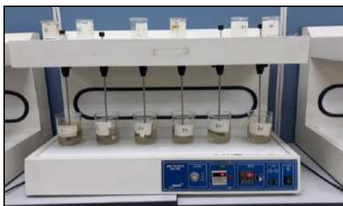
Figure 2: Jar Test Method for both coagulants alum and natural in IUKL Laboratory
