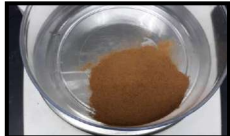
Figure 6: The kernel after grinded and sieved
