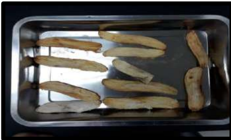
Figure 5: The kernel has been extracted after 24 hours oven dried at 105°C
