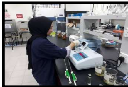
Figure 11: Turbidity results were recorded by using Turbidimeter
