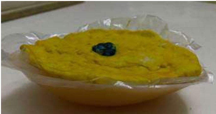
Figure 7: Developed homogenous breast phantom with tumour
