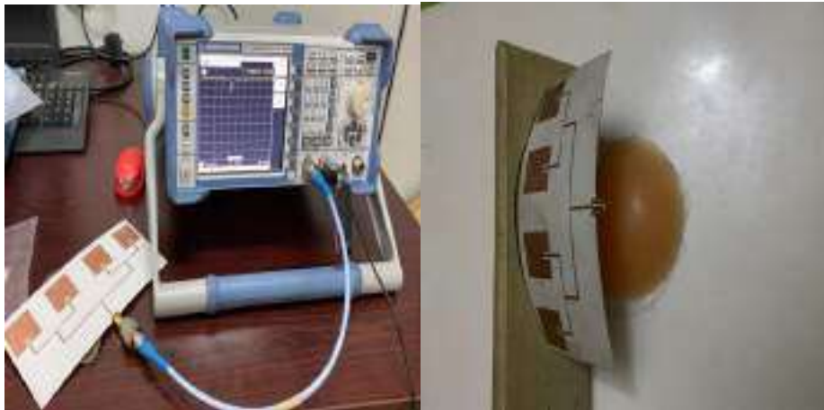
Figure 8: The Experimental setup. (a) Breast phantom under the antenna array after the antenna has been set up with vector network analyser. (b) presents how the antenna array is bent around the breast phantom
