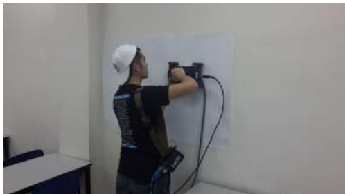
Figure 5: GPR Scanning On Area 3 (Wall)
