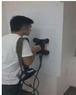
Figure 6: GPR Scanning On Area 4 (Column)
