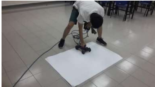
Figure 4: GPR Scanning On Area 2 (Floor)
