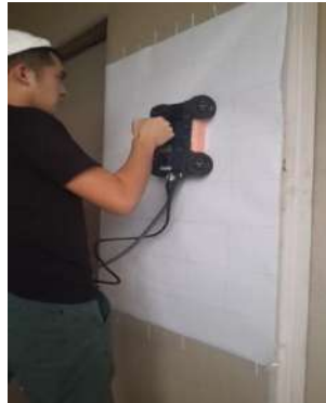
Figure 8: GPR Scanning On Area 6 (Column)
