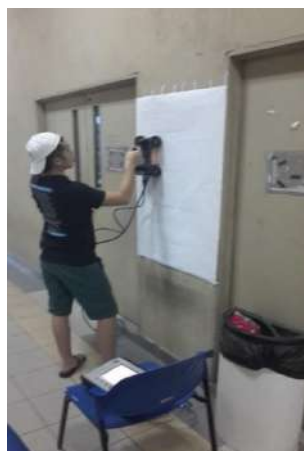
Figure 7: GPR Scanning On Area 5 (Column)
