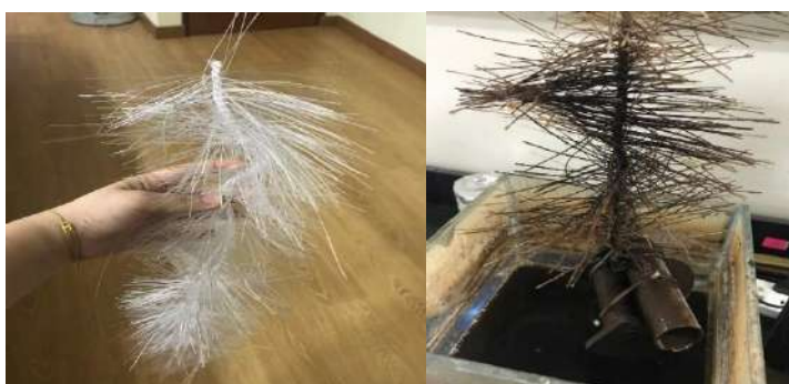
Figure 2: Colour of Attached Growth Media Changed from White Colour to Brownish Colour
