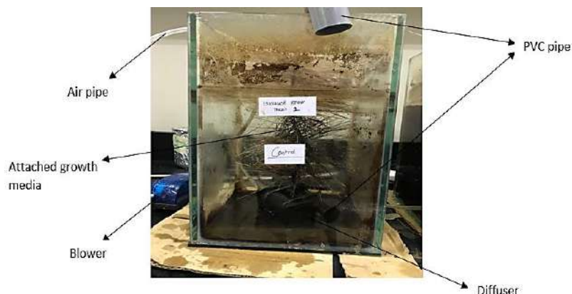
Figure 3: Lab Scale Set-up Represented as Conventional Attached Growth System
