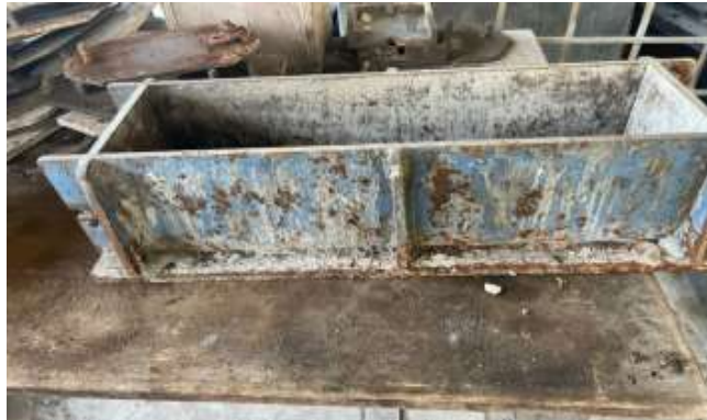
Figure 3: Beam mould 150 x 150 x 500m
