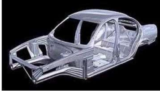
Figure 1: Monocoque Chassis ( Mark Wan,2000 ).
