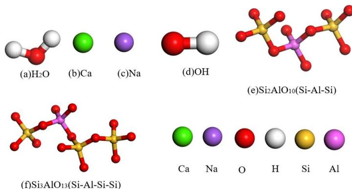
Figure 1: The basic unit of geopolymer gels
