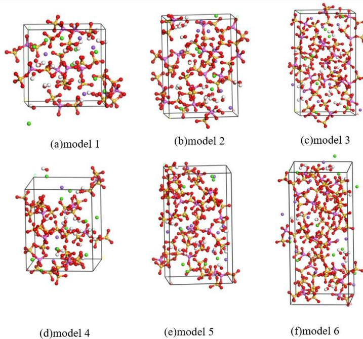
Figure 2: The structure model of geopolymer gel
